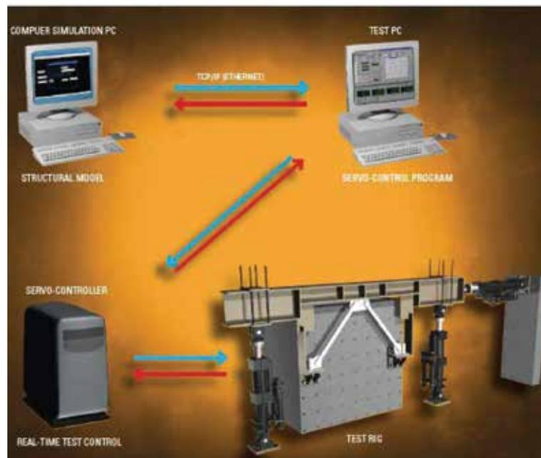
Quasi-static Hybrid Simulation System Diagram
