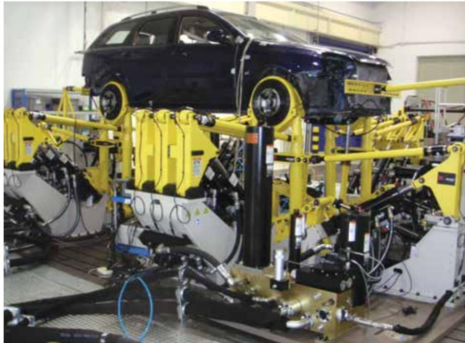
capabilities. It installed several sets of vehicle road simulation test beds, a simulation test platform (MAST), a small 3DOF vibration table composed of various actuator cylinders, a suspension test bed, a steering gear test bed and more. This wide array of equipment has also enabled the PAATC to develop a very well-trained staff of testing technicians.
