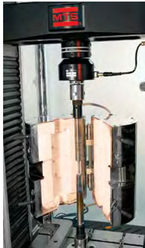
MTS Fundamental Furnace
