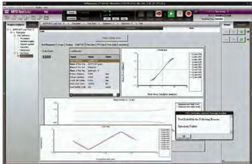
The Runtime View provides a comprehensive view of HCF tests in progress, including hysteresis loops, displacement peak and valley per cycle, and load-time trace per cycle.
