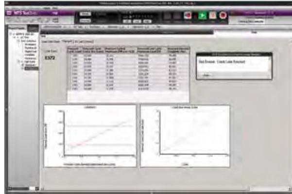
The Runtime View of the pre-crack portion of the J<sub>Ic</sub> test can simultaneously display tabular results per cycle, load versus COD, and crack size versus cycles.
